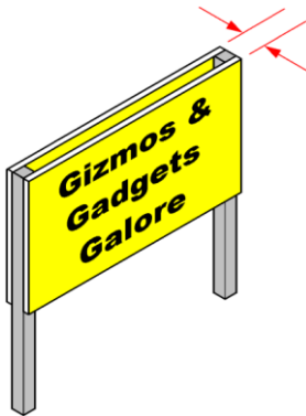
Figure 3.10C – Sign Faces Less than 30 Degrees Apart
