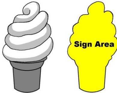
Figure 3.10E – Area of a Three-Dimensional Sign
