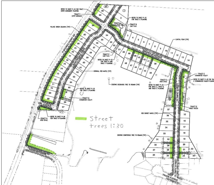
Exhibit PUD-3h: Site Plan Sheet P-31 Street Tree Min No. (green: equal to 1 tree per 30 ft of block frontage)
