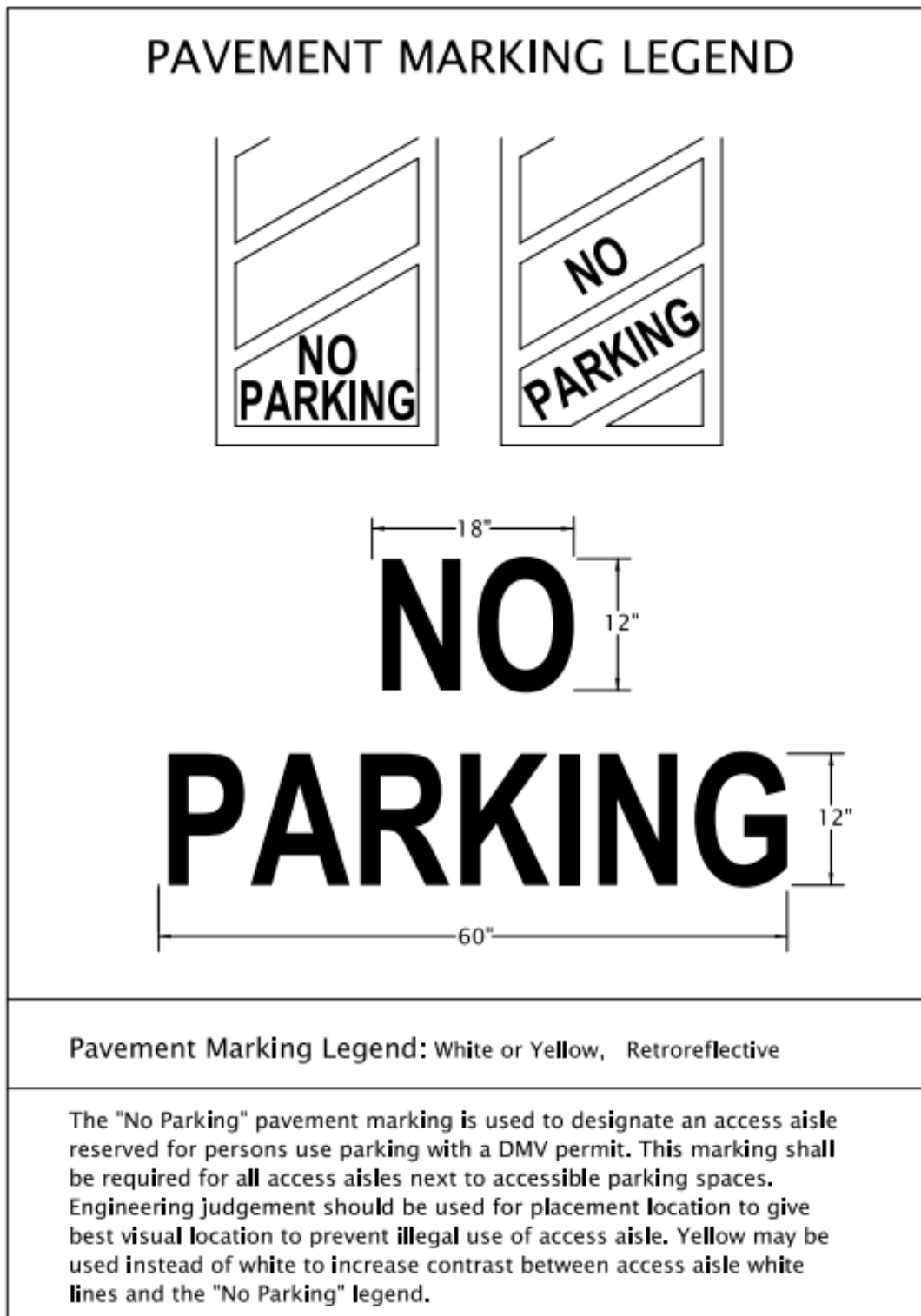
Figure 7: Pavement Marking Legend details for NO PARKING
