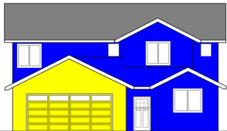
Figure 3.107B – Garage (yellow) comprises no more than 65 percent of total facade (yellow plus blue)
