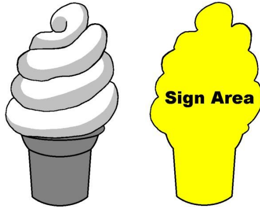
Figure 3.10E – Area of a Three-Dimensional Sign
