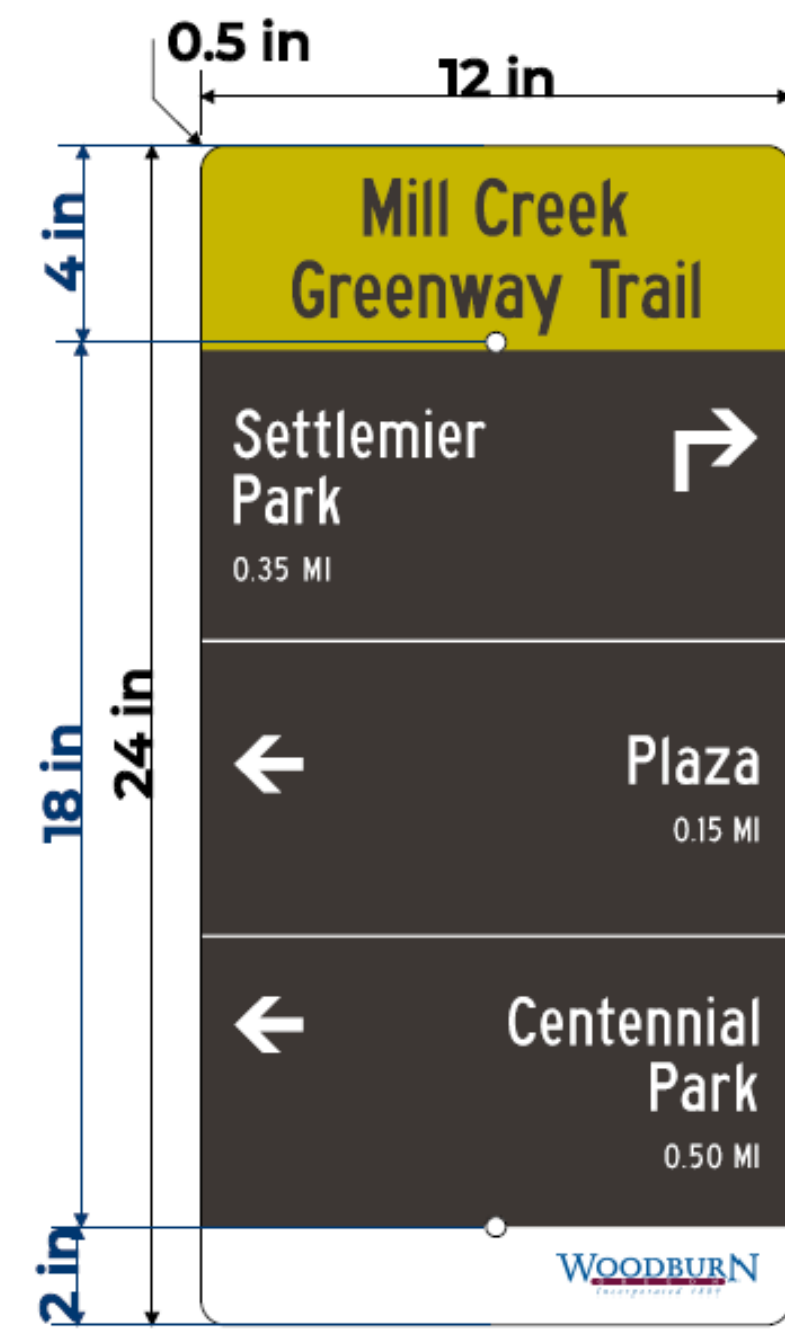
TYPICAL WAYFINDING SIGN NOT TO SCALE
