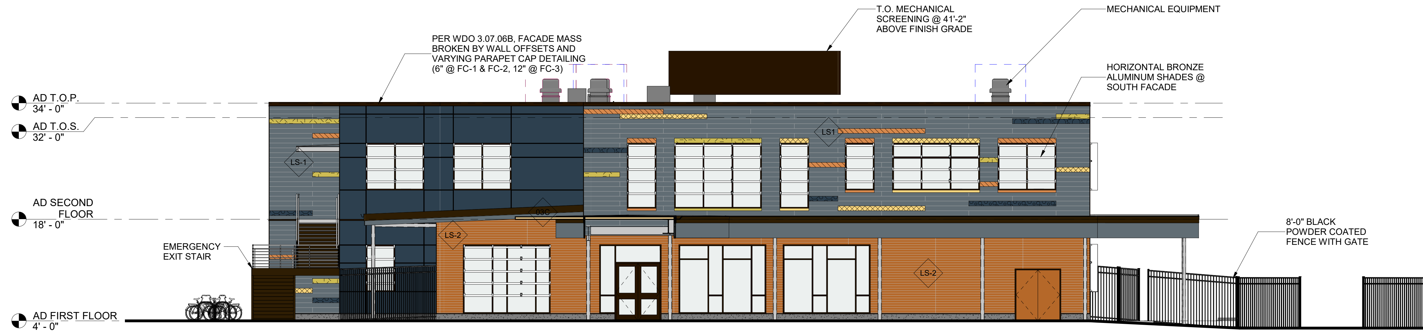
3 SOUTH ELEVATION - ZONE A - CONDITIONAL USE 1/8" = 1'-0"
