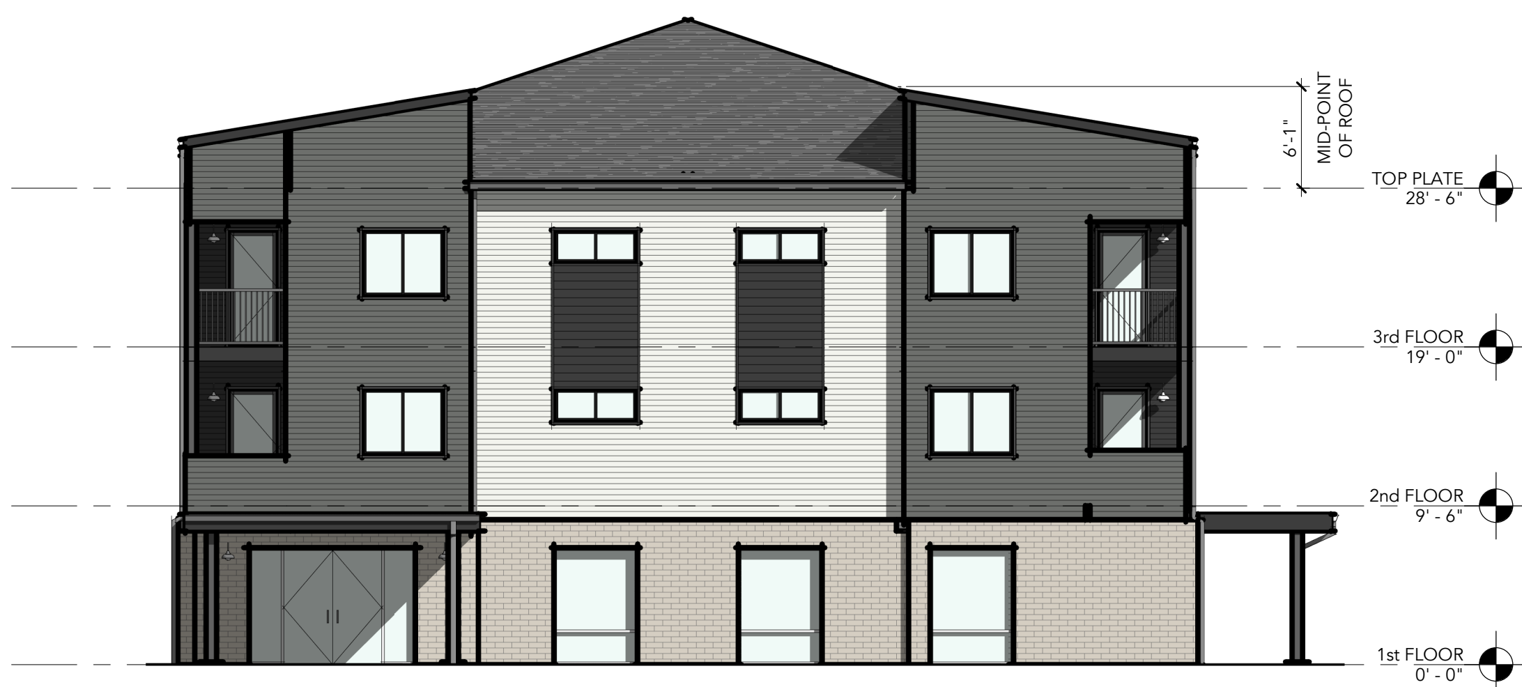
2 SIDE ELEVATION (LEASING BUILDING) SCALE: 1/8" = 1'-0"
