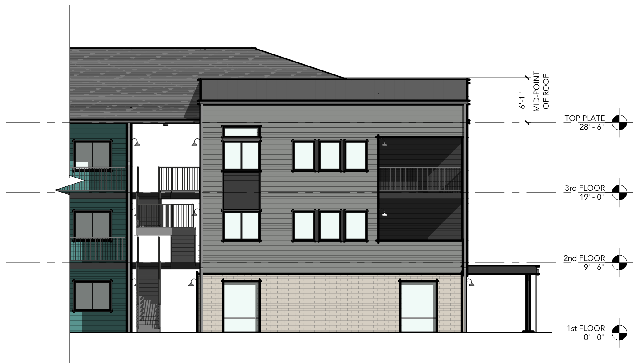
3 PARTIAL BACK ELEVATION (LEASING) SCALE: 1/8" = 1'-0"
