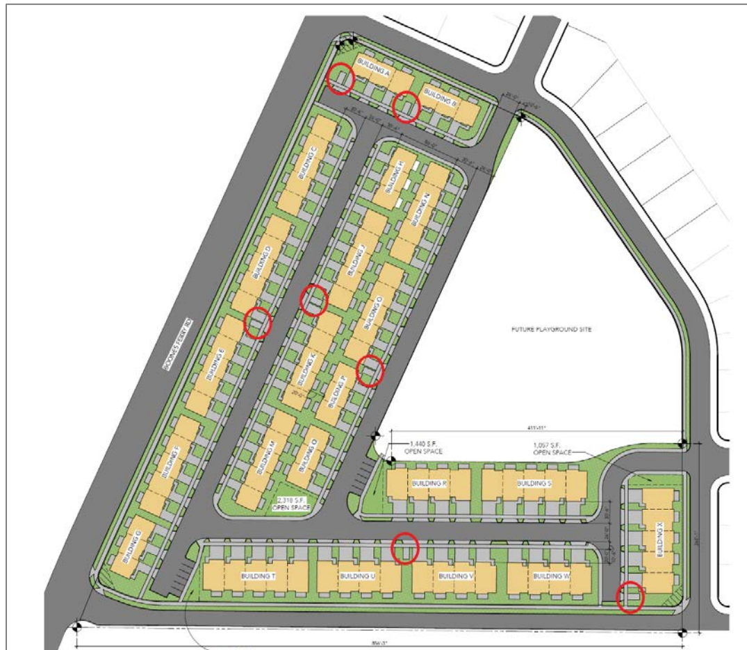
Revised site plan with parking stalls to remove and replace with landscaping circled in red.
