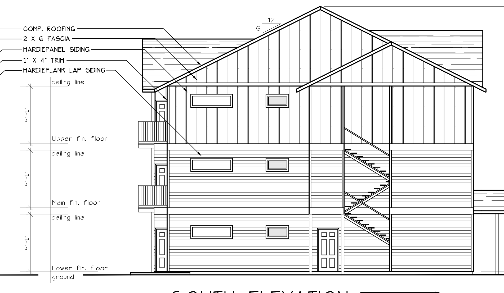
SOUTH ELEVATION (TYPE D UNITS) SCALE: 1/8" = 1'-0" BLD. 1
