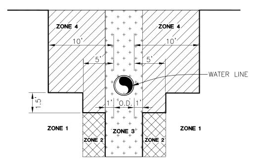
ZONE 1 SEWER LINE BE LAID IN THIS AREA WITH NO SPECIAL REQUIREMENTS OF EITHER CONSTRUCTION OR MATERIALS OTHER THAN THOSE SPECIFIED.
