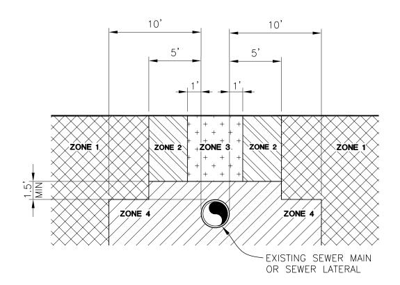
ZONE 1 XXXX WATER LINE CAN BE LAID IN THIS AREA WITH NO SPECIAL REQUIREMENTS OF EITHER CONSTRUCTION OR MATERIALS OTHER THAN THOSE SPECIFIED. CROSSING RESTRICTIONS SHALL APPLY.
