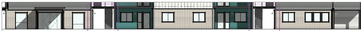
Excerpt of elevations: Building A ground floor that faces Young Street. Purple outline indicates breezeways and stairwells.
